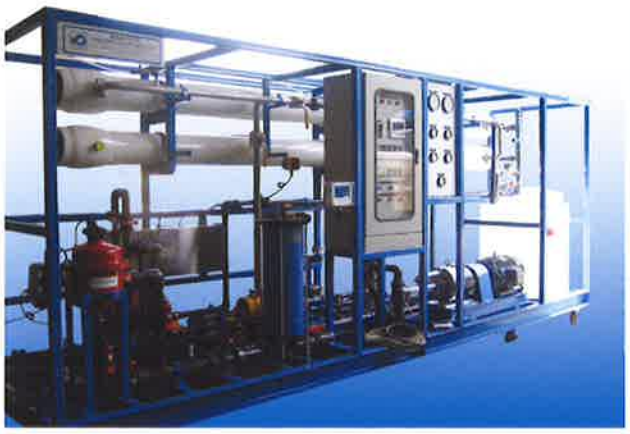
100,000 litres/day production capacity Seawater RO powered completely by solar power in Abu Dhabi, UAE
