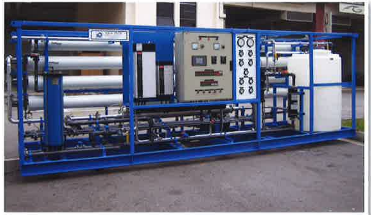
200,000 litres/day production capacity Seawater RO with PX Energy Recovery Device in Zanzibar, Tanzania
