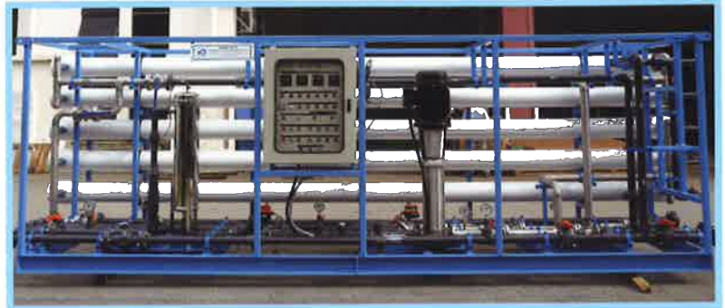
500,000 litres/day capacity MBR-RO in Abu Dhabi, UAE
