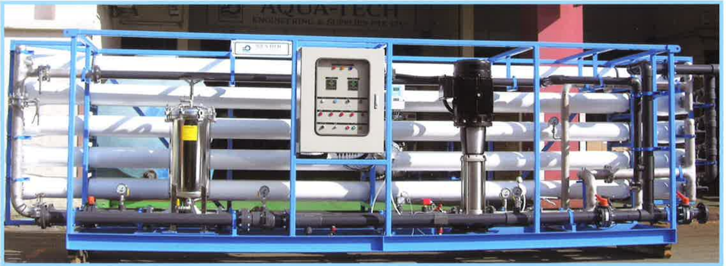
1,000,000 litres/day production capacity MBR-RO in Dubai, UAE
